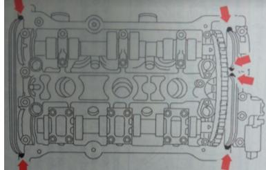
Apply sealant (Ajusil) in the transition area of the caps in the cylinder head as shown in the repair manual.
