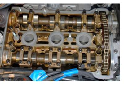
Clean all surfaces before installing the new gasket. Install the new gasket with special attention where the gasket fits into the slots on the sides of the cylinder head.
